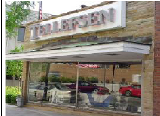
Pin-mounted letters on an obtrusive box that projects from the storefront (2b)
